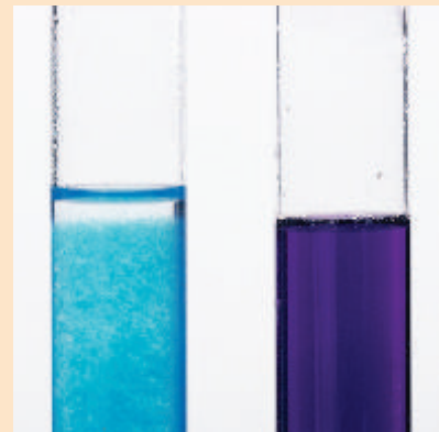
Figure 3.8 Results of the Biuret test for proteins
